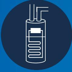
**With a patented aluminium heat exchanger,** Edel transfers a higher amount of energy compared to traditional copper wound heat exchangers
